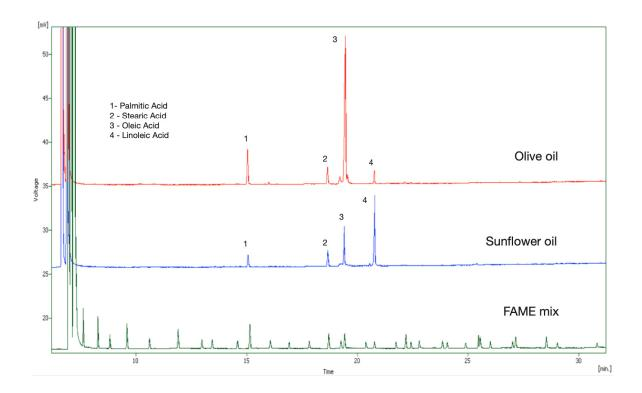
Column used - ELR-CN100 60 m x 0.25 mm x 0.20 um film thickness
